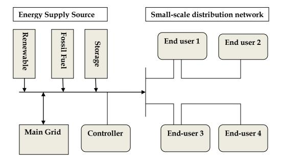
Storage is required to cope with the variable and uncertain output that is characteristic of renewable energy sources. Storage is critical even for main-grid connected mini-grids if they are expected to support essential services when there is a breakdown of the main-grid. In developed countries which have achieved universal access there is increased interest in mini-grids because of this ability to provide supply to essential services such as hospitals during emergencies.
